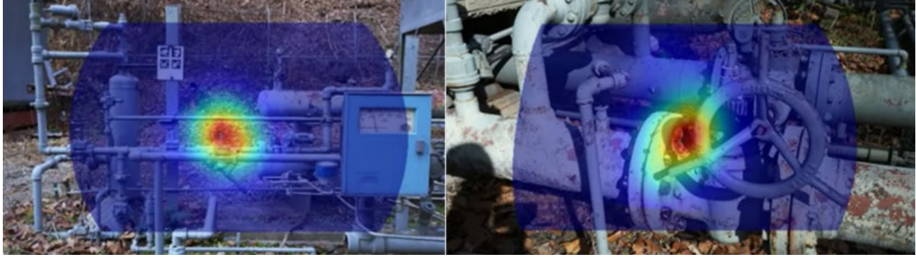
Figure 7. Examples of component-level emission source detection in oil and gas facilities recorded from distances of 3 meters and 1 meter.
