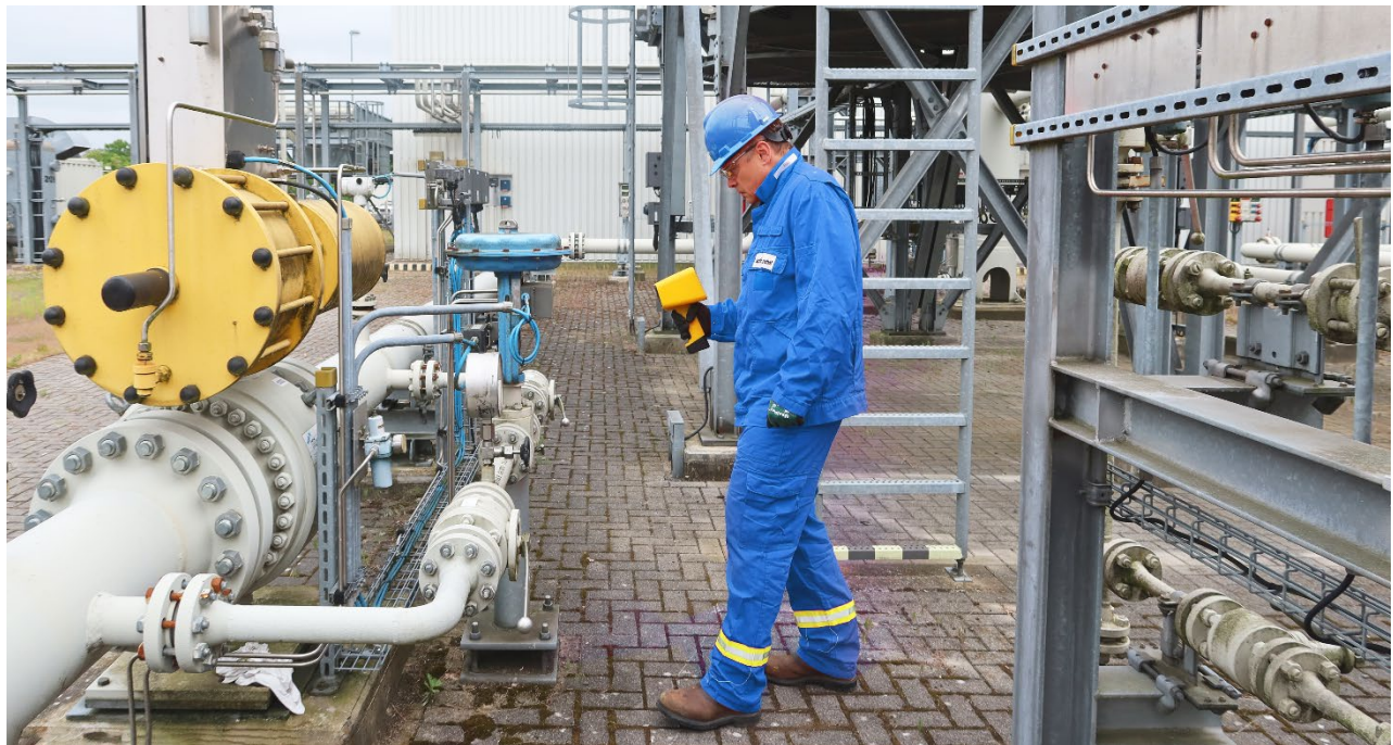
Figure 9. Scanning equipment and components with Xplorobot Laser OGI device.
